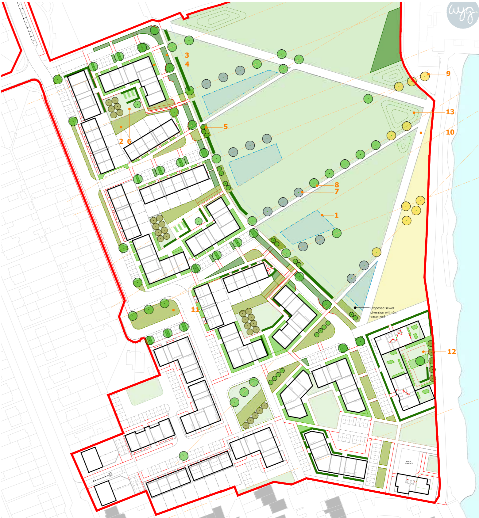
Highlight SuDS processes through decorative markers across footpaths Online SuDS ponds withing localised deepening of detention basins to increase biodiversity The Marl SuDS and development edge treatment to provide separation Footpath edge rill to extend SuDS through hard landscape Wetland with informal play opportunities along edges to form a Rain Park Rain park signage Limited Permeable Paving where there is no 'green' alternative SuDS linked through hard landscape and Living Streets Annual meadow transition space into The Marl and SuDS basins Rain garden build outs within Living Streets and traffic calming
